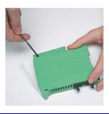
Using a small flat head screwdriver release all four of the enclosure cover hooks.
