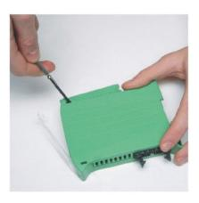
Using a small flat head screwdriver release all four of the enclosure cover hooks.
